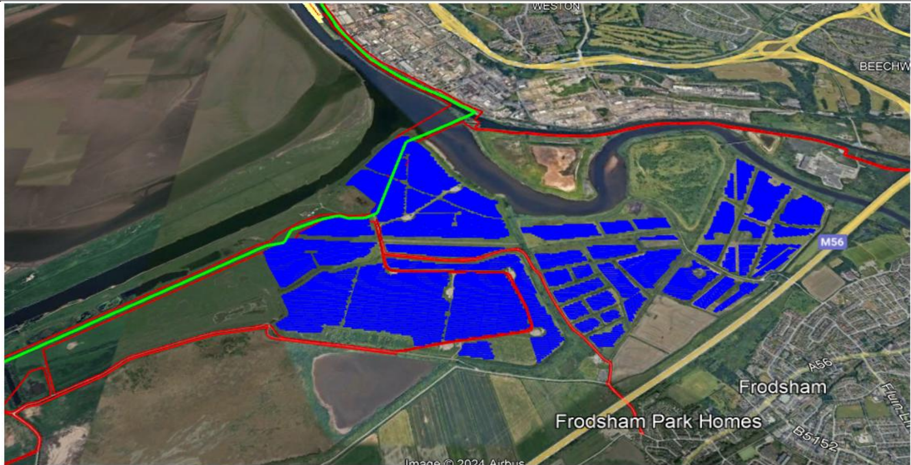
Figure 3 - Outlined Interaction of Runcorn Spur CO2 pipeline with Frodsham Solar Development (latest proposal)
